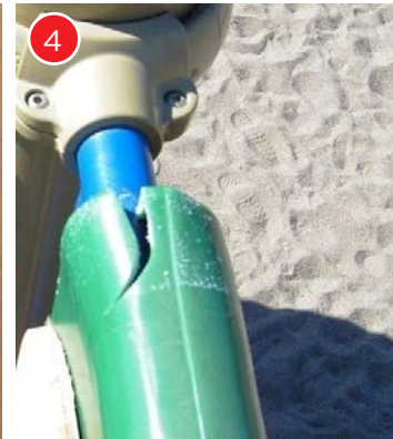
This cracked component is a hazard.
